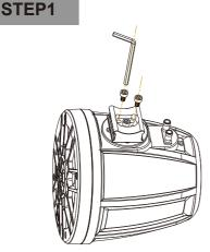
The two screws can be unbolted to loosen the metal base of the mounting band to adjust the mounting angle. Make sure to put all components of the mounting hardwares in a safe location.
