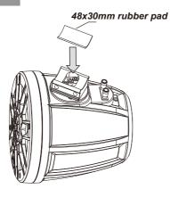
Place the front rubber pad on the metal base of the mounting band.
