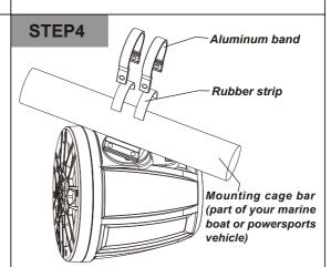
Place the supplied rubber strip around the cage bar to prevent scratching. Push the aluminum band over the cage bar. Align the aluminum bands with the metal base of mounting bands on the waketower speaker.
