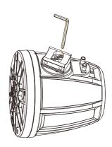
After loosening the two screws and determining the optimal angle for your speakers on the mounting cage, tighten the two screws in place to secure the metal base of mounting band tightly.
